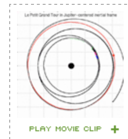
Petit Grand Tour trajectory seen projected onto the orbital plane of Europa and Ganymede
